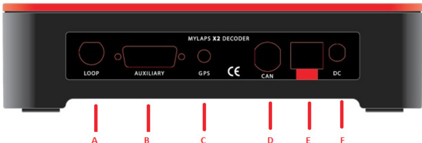
Figure 1.2 Connections of the decoder
